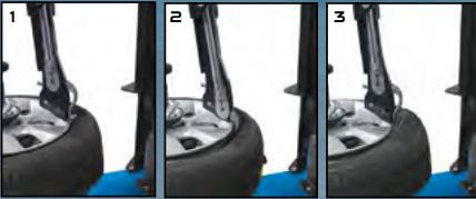
Evolution Device to convert standard machine into leverless operation
