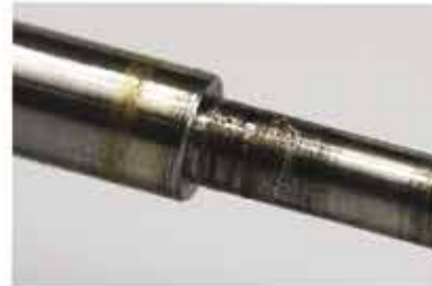
shaft discolouration due to oil starvation
