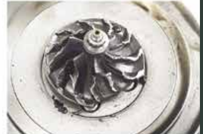
foreign object damage to compressor wheel
